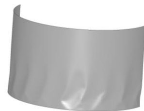
Tsunami-induced buckling of tank
