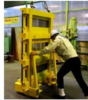
Portable Radiation Shielding Apparatus: Mobile Shield MRS® (developed in-house)
